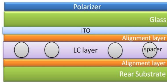
Figure 2.3 The cross-sectional profile of a reflective MTN-LC cell.
